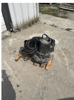
Left: Scum beach being repaired, Right: 3" trash pump used for proof-of-concept testing
