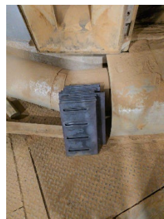
Left: Teeth extensions fabricated and ready for install Right: Teeth extensions installed on rabble teeth
