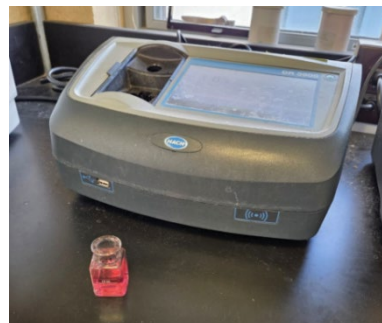
DR3900 with a sample ready to be tested
