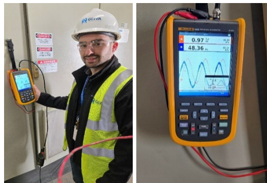
Power Management Professional Nick Romund using the Fluke 125B and the display on the screen
