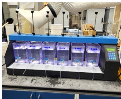
Jar testing at Water Works Park
