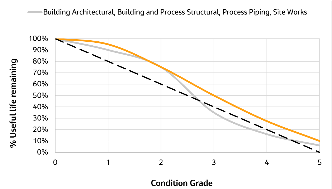
Figure K-2: Condition-based deterioration curves
