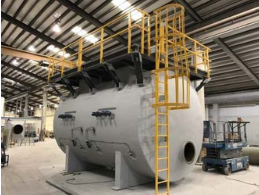
Figure 7-7. Example of Ladder, Platform and Railing (figure is not Belle Isle's odor control system)
