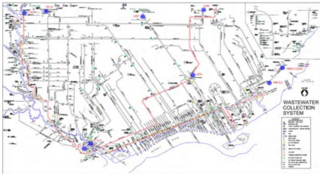
Figure 1: New Level Sensor locations to measure hydraulic grade level downstream of Member meters
