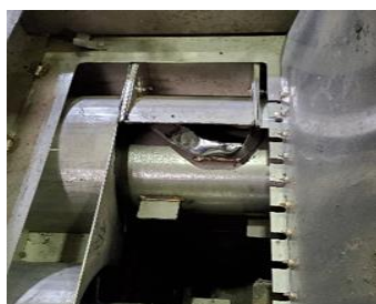
Liner Restraint Jammed Chute from H to K Belt overloaded In Screw Hopper 14B (Photo shown left)
