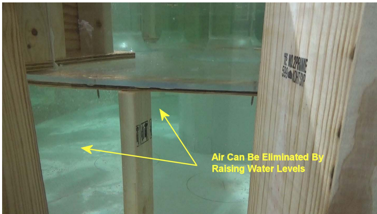
Photo 5-5 Revised Water Levels Minimize Air Entrainment
