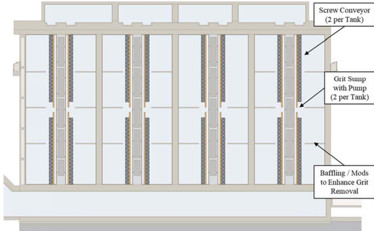
Figure 6-10: Layout of the Rehabilitation of the Aerated Grit Chambers with Screw Conveyors
