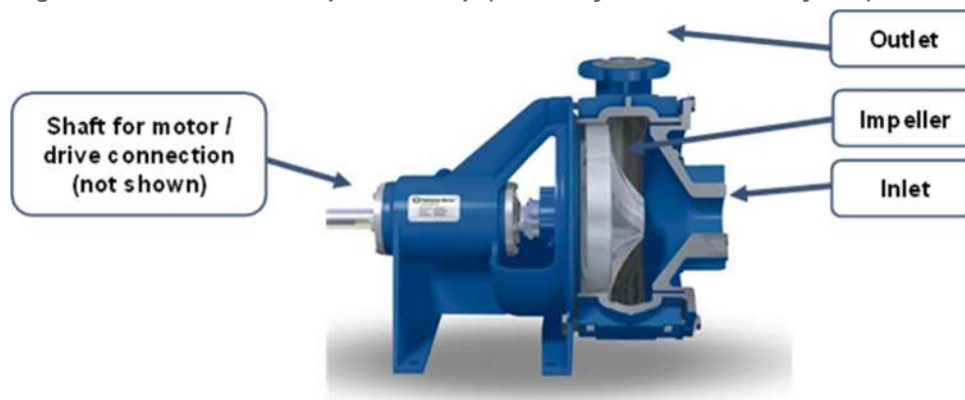
Figure 6-24: Recessed Impeller Pump (Courtesy of Fairbanks Nijhuis)
