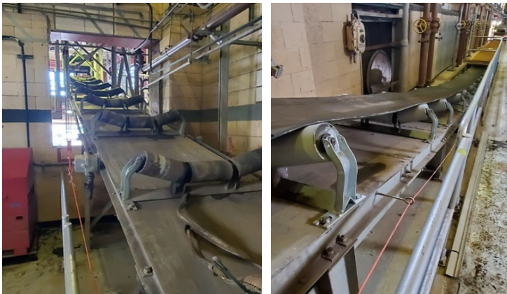
The old rollers and belts were replaced for the sky belt before a critical failure.
