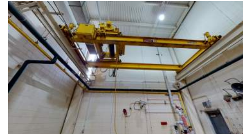
Corroded building crane from failed HVAC system
