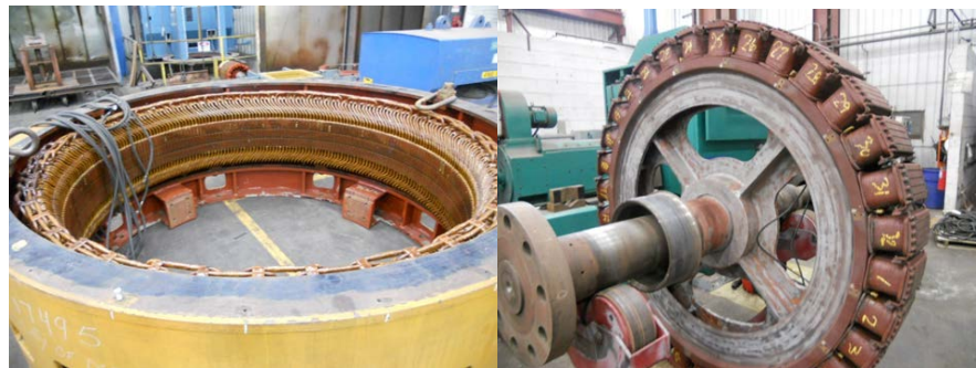
Images of Manlift pump #5 repairs of the stator (image on the left) and rotor
