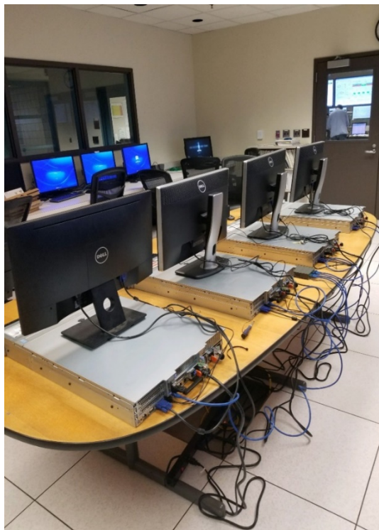
New Ovation Process Historian and Domain Controllers preparation
