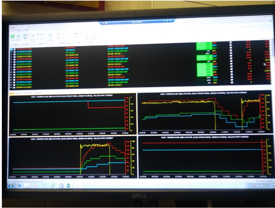
Pre-Built Trend for Main Lift Pumps 1 THRU 4
