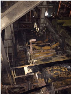
Picture from left to right Sludge Conveyor G Damaged by Fire and Conveyor B in the Complex – II Dewatering Building and Fire Damaged Conveyor H in Complex-II Incinerators Building
