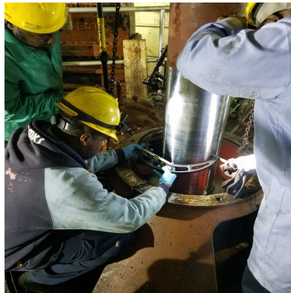
Primary Team Members measuring a shaft diameter
