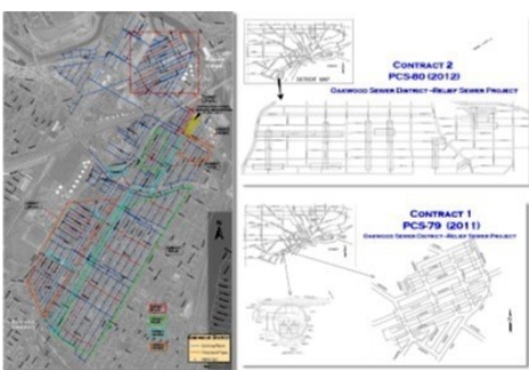
Aerial photo, far left, of Oakwood Sewer District depicting previously designed relief sewers tributary to Oakwood Pump Station and CSO Retention Treatment Basin. Part of the planned relief sewers and associated hydraulic structures were constructed between
