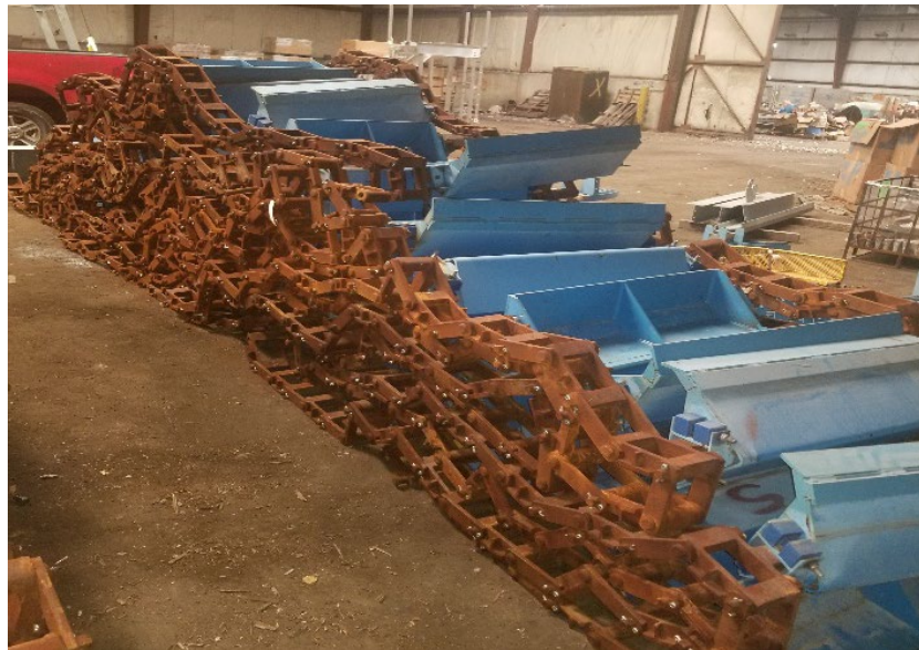
Replacement grit channel chain and buckets
