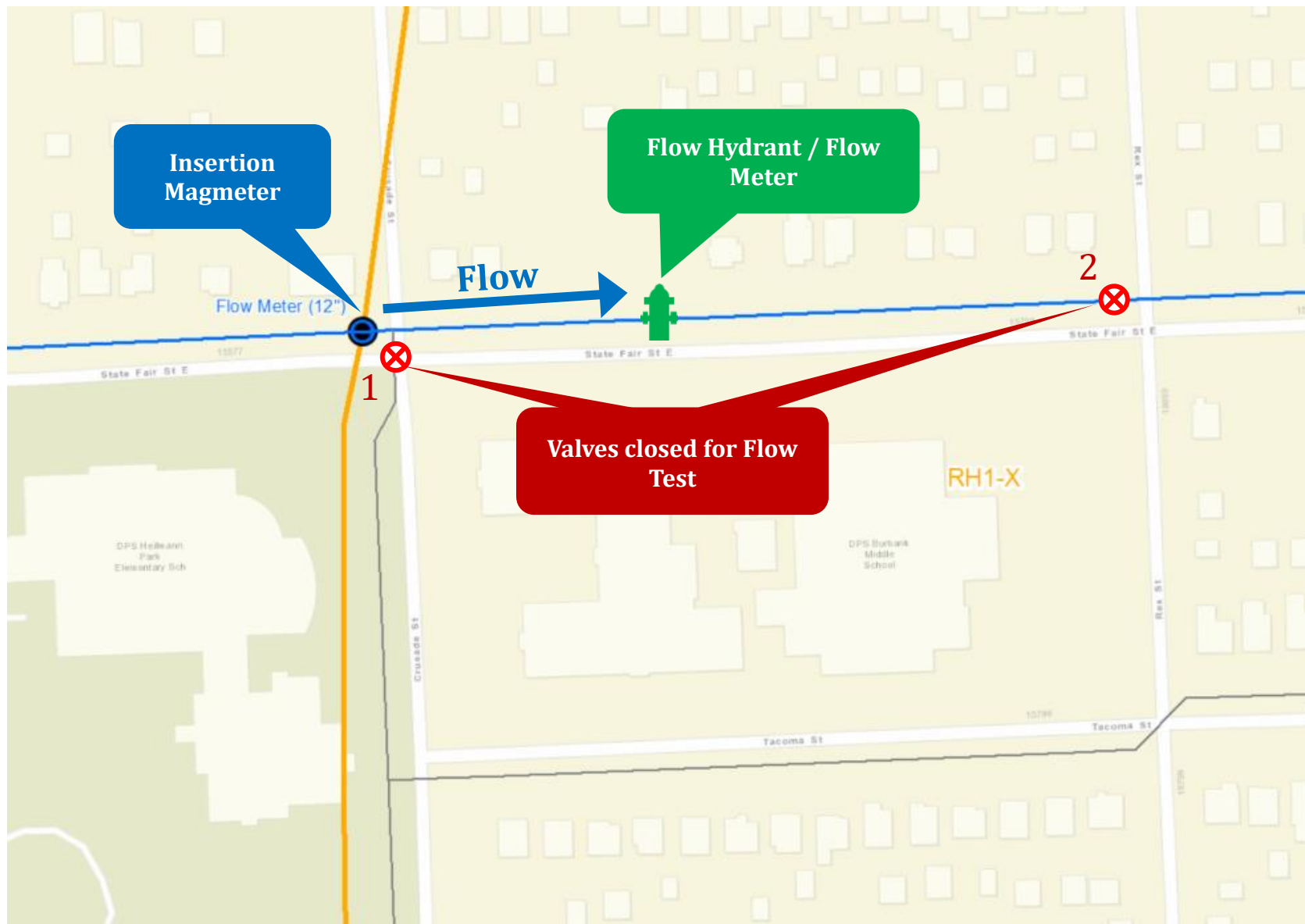
Figure 9-7 In-Situ Flow Test on State Fair St. E Meter
