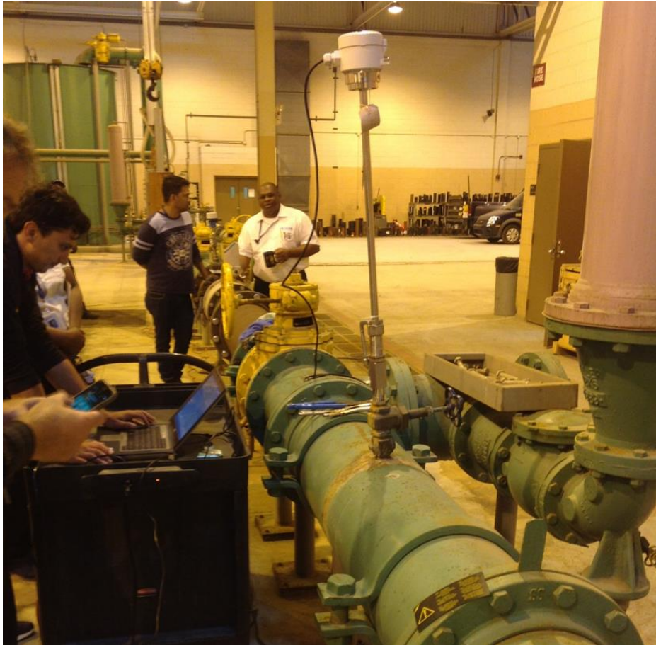
Figure 2-20 Insertion Flow Meter Test Bench Configuration
