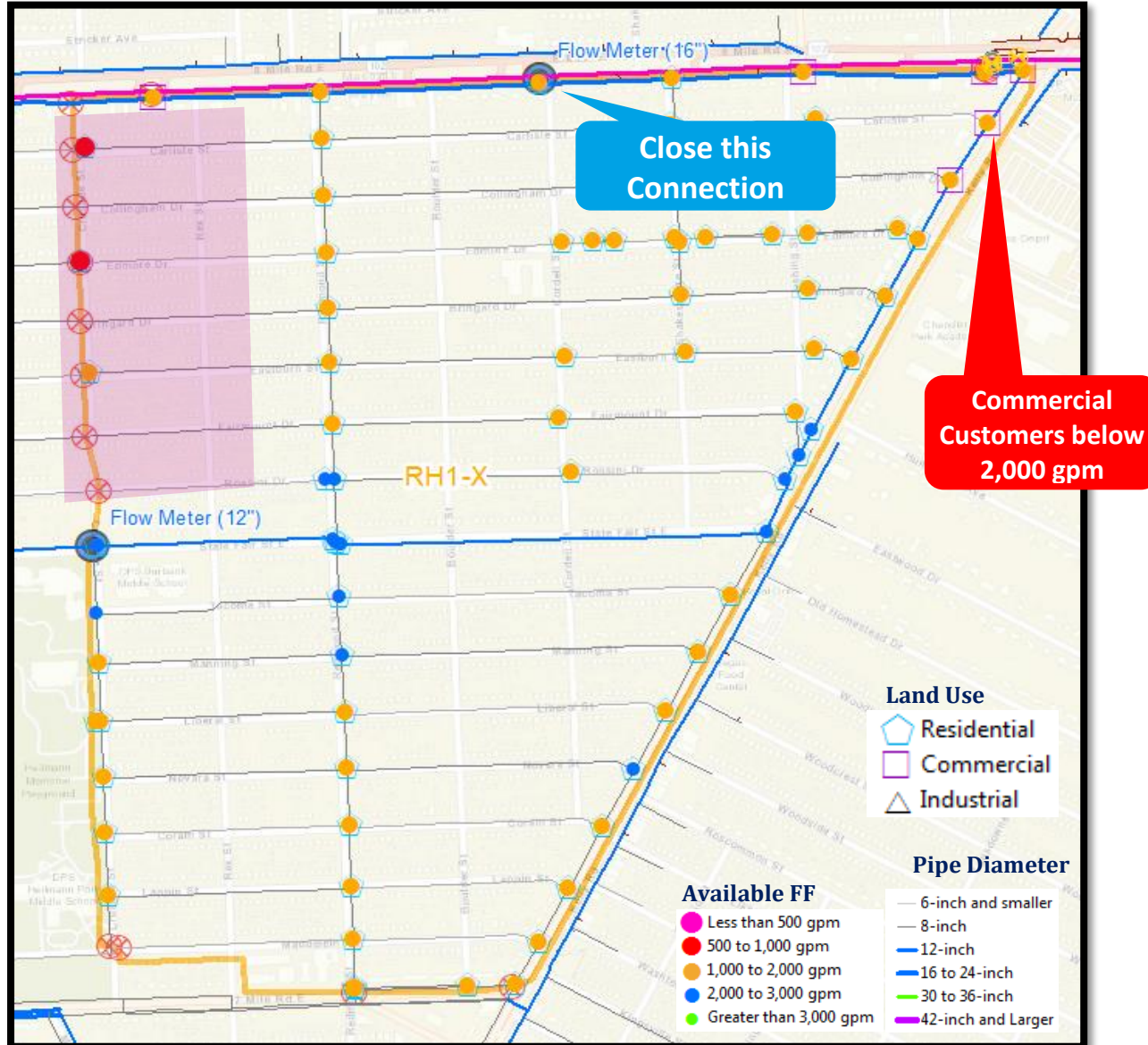
Figure 9-6 RH1-X Fire Flow Planning (One Input Scenario)
