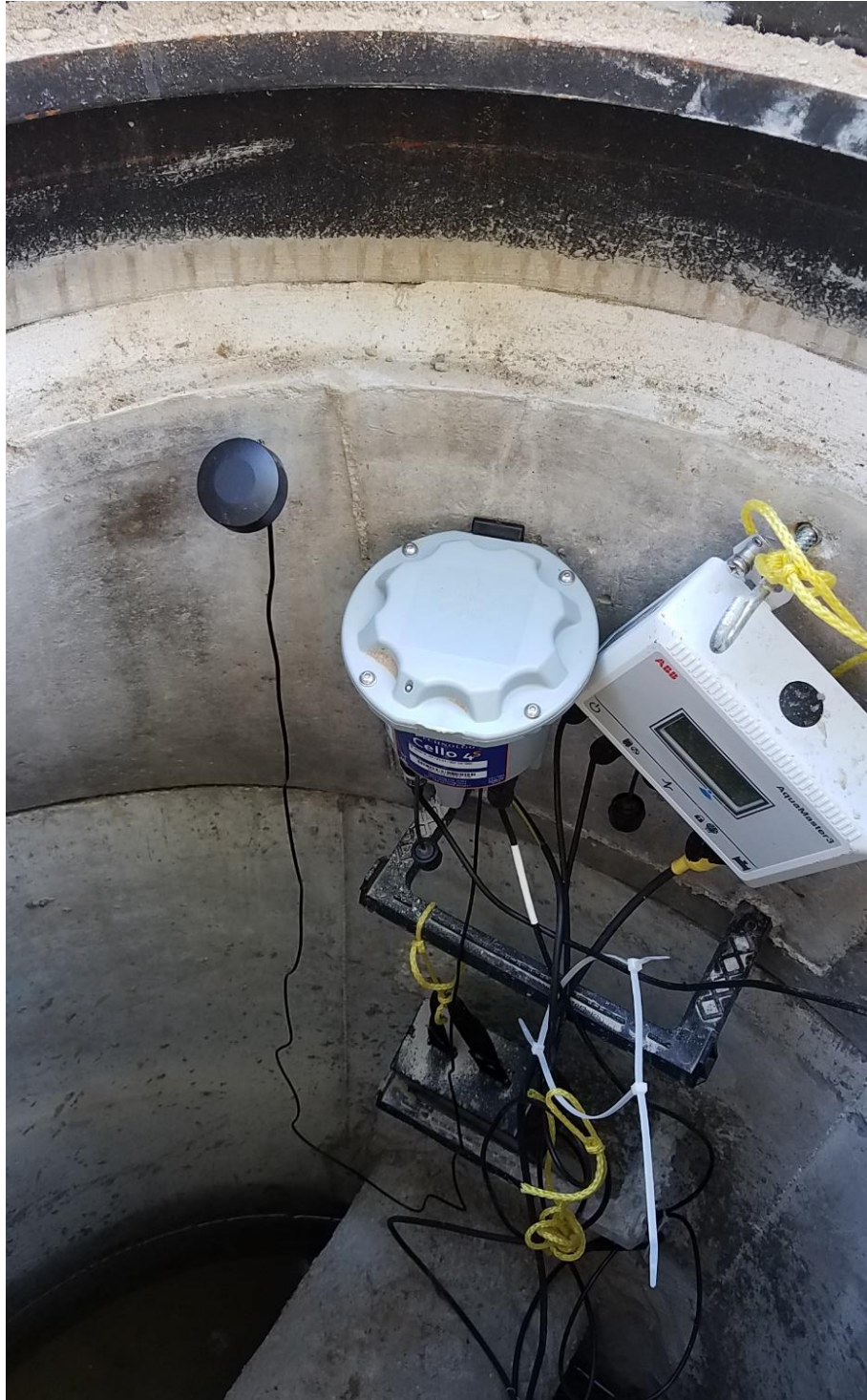
Figure 2-23 Example Installation of Flow Logging Infrastructure (from DB1)
