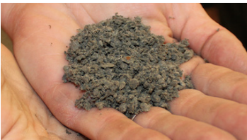
Fertilizer pellets created by the Biosolids Dryer Facility
