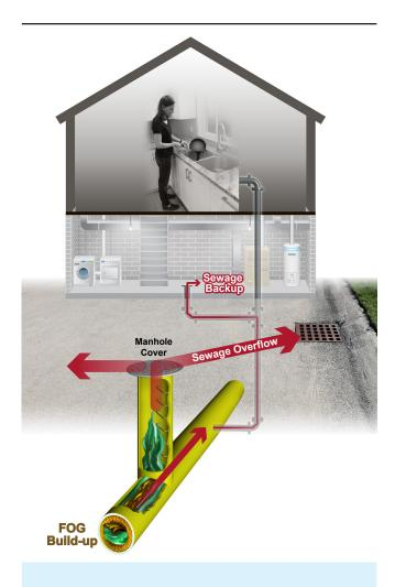
FOG enters sewer pipes through restaurant, residential and commercial sink drains. Once in the sewer. FOG sticks to the pipe and thickens. FOG can build up and eventually block the pipe and send sewage backward out of manholes into streets and rivers, or up floor drains into homes.
